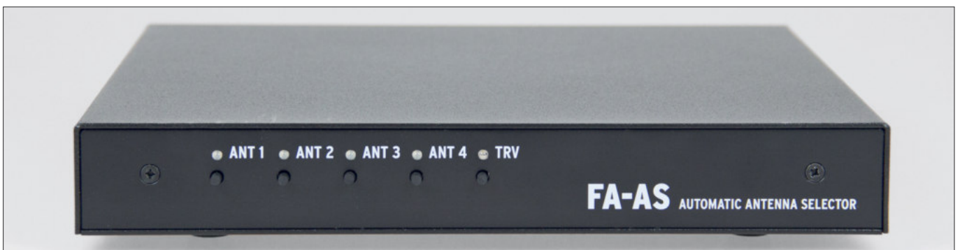
Picture 1a. Front view of the fully built FA-AS
