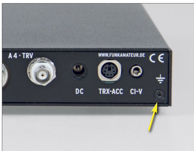
Picture 25. Rear view of the fully built FA-AS; the earth symbol marks the housing screw which serves as the earthing point.
