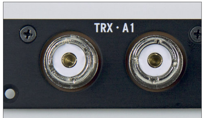
Picture 16. The five SO 239 sockets should be mounted such that they are centred in the holes on the rear panel.
